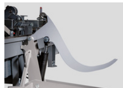
Additional arm to the log loader 1000
