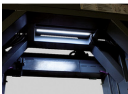
LED lighting (11 W)
